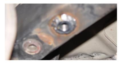
Once satisfied with the fitment of the bungs weld the bungs to the frame. Remove any bolts installed and allow welded area to thoroughly cool before proceeding.
