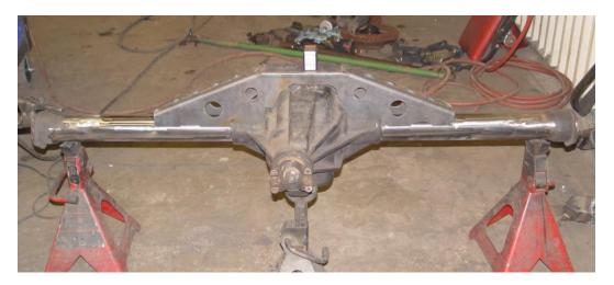
**CAUTION:** Welding operations should be performed by a qualified technician. TNT highly recommends that the truss assy. be stitch welded in place. You should only weld in 1" increments and the truss/axle tube should be cool to the touch before welding again.
