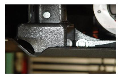
**NOTE:** Do not tighten fasters at this time, you will need to position the Xmbr side to side to center it under the Jeep's frame. The XD Xmbr may angle down from the back of the XD Belly Pan slightly. This is normal and is part of the overall design.
