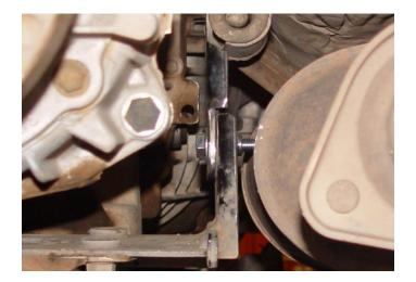
**STEP 4:** Raise your TNT bellyskid into place, be sure to align transmission mount and temporarily bolt to the frame using two  $\frac{1}{2}$ " bolts from the supplied hardware (12mm bolts on 03' & newer models).
