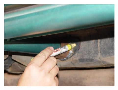
Remove the rail assembly from the vehicle and drill the mounting cups bolt holes that you just marked with an 11/32" drill bit.
