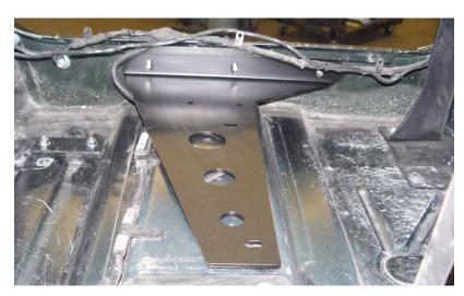
**STEP 3:** Reinstall seat bolts, and the remaining slider mounting bolts. Tighten all fasteners.
