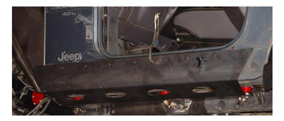
**STEP 4:** Mark the upper mounting holes on the body using a marker or transfer punch. Remove the Rocker Guard and set it aside.
