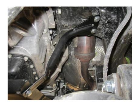
**Step 4:** Select 4-5/16" X 1" bolts and clip nuts from the hardware kit. Install clip nuts in factory holes at engine motor mounts so that bolts can be installed facing up. Secure the struts to the frame side of the engine.
