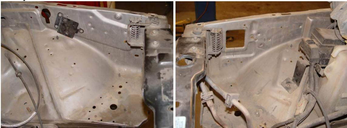
**STEP 2: Factory Inner fender Removal**
