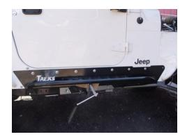
**STEP 6:** Mark the upper mounting holes on the body using a marker or transfer punch. Remove the Rocker Guard and set it aside.
