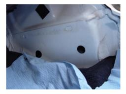
**STEP 8:** Reinstall the Rocker Guard. Install the 3/8" hardware supplied, tighten to 30 ft-lbs.
