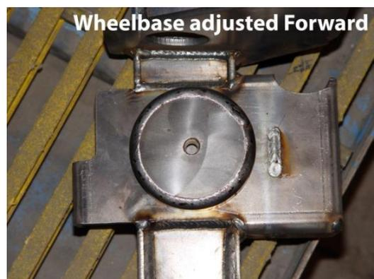
Once the desired location of the cup has been achieved, center cup side to side, tack weld into place. Repeat steps for passenger side cup. Install coils and control arms, verify fitment of components. If satisfied, remove coils and weld caps approximately 1" across front and 1" across the rear.
