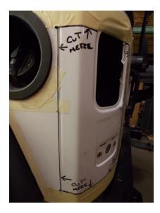
7. Cut out the marked areas to remove the factory raised sheet metal.
