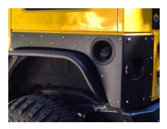
8. Place the driver's side Guardian™ Corner over the corner of the Jeep. The Guardian™ Corner will slip snugly over the fuel filler trim piece, helping to align the corner. Ensure that the distance between the top edge of the Guardian™ Corner and the top edge of the Jeep's tub is the same from front to back. When happy with the alignment securely clamp the Guardian™ Corner into place.
