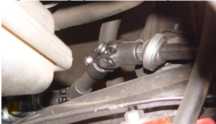
Fig. 4 – Steering U-joint & heim assembly
